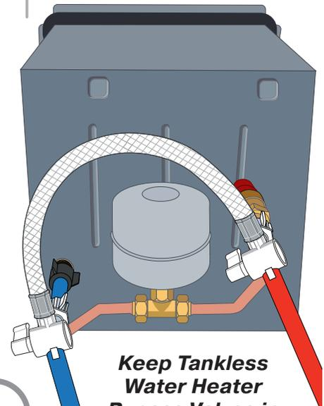
**Keep Tankless Water Heater Bypass Valves in the Normal Position**
