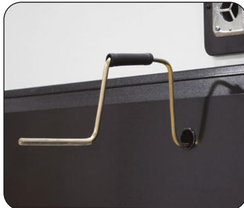
*Slideout Override Access Hole & Crank Handle Extension*
