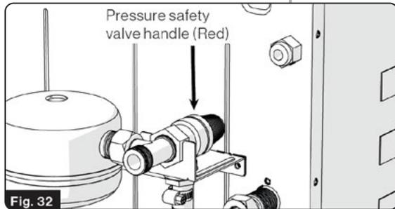
8. Inspect the pressure safety valve to ensure it has not been leaking (no water residue). See "Pressure Safety Valve Maintenance" for further inspection. (Fig. 32)
