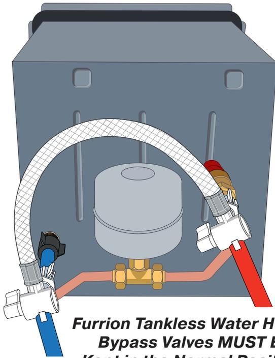
**Furrion Tankless Water Heater Bypass Valves MUST Be Kept in the Normal Position.**
