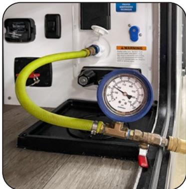
Air Compressor Hose with Pressure Gauge
