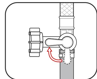
**Normal Use** Bypass Valve Position is used for Draining the Water Heater:
