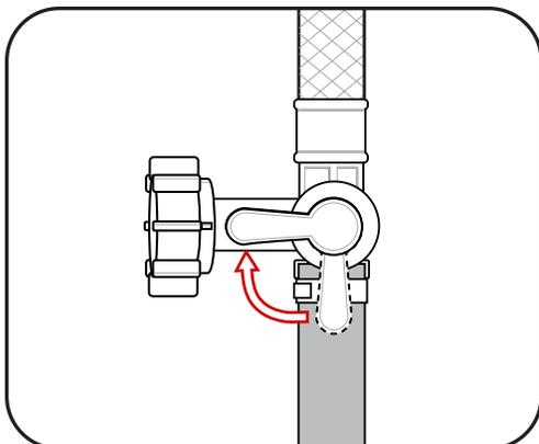
**TURN BOTH** bypass valve handles towards the water heater.
