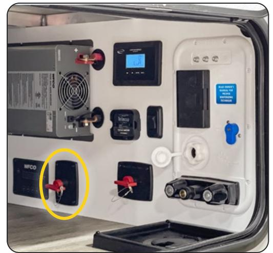
2000 Watt Inverter & 2nd Battery Disconnect
