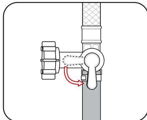
**TURN BOTH** bypass valve handles towards the hot & cold water lines.
