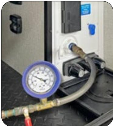
Air Compressor Hose with Pressure Gauge
