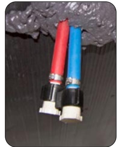
*Low-Point Drain Valves located under the RV*
