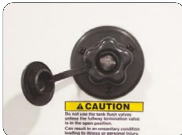
*The Black Tank Flusher Inlet is located on the off-door side of the RV.*
