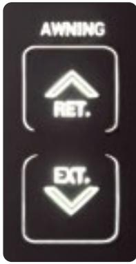
The Patio Awning Switch is located inside the RV, on the Command Center
