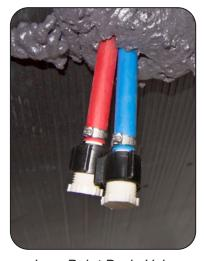
Low-Point Drain Valves located under the RV
