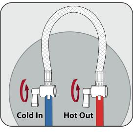
6-Gallon Water Heater Bypass Valves.
