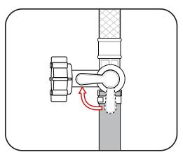
TURN BOTH bypass valve handles towards the water heater.
