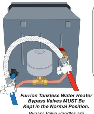
Bypass Valve Handles are Shown in Normal Use Position.
