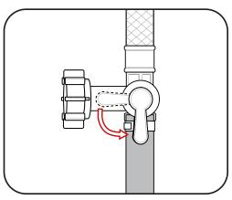
TURN BOTH bypass valve handles towards the hot & cold water lines.
