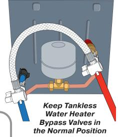
(Bypass Valve Handles Turned Towards The Water Heater)
