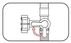
When Winterizing or Sanitizing the 6 Gallon Water Heater, use the Bypass position. TURN BOTH bypass valve handles towards the hot & cold water lines as shown:
