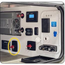
2000 Watt Inverter & 2nd Battery Disconnect
