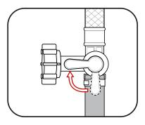
**Normal Use** Bypass Valve Position is used for Draining the Water Heater:
