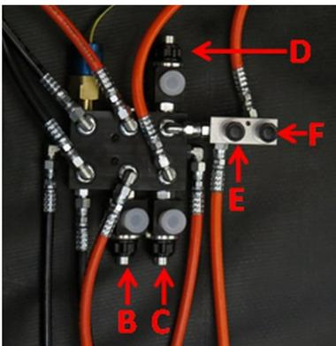
Typical hydraulic slide rooms and leveling legs override valves, generally located in the front facing compartment.
