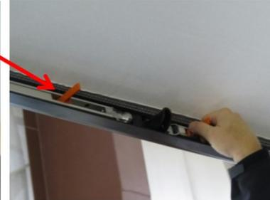
2. Locate both orange colored locking mechanisms at the top inside of the extended awning, and pull the handles towards you (as shown above) to release the retractable legs.
