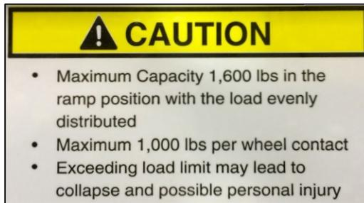
*Follow the above weight label instructions when the ramp door is in the ramp position.*
