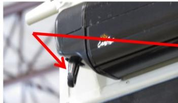
1. Locate the turning mechanism located on the rear awning, then insert & rotate the awning handle to manually extend the awning. Stop when the awning is fully extended.
