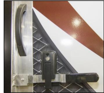
*Photo shows typical ramp door handle and lockset*
