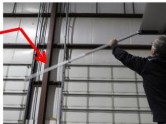
3. Next, push the orange colored handles outwards to release the retractable legs (Tip: rotate the retractable legs downwards as you push the handles out, as shown above).
