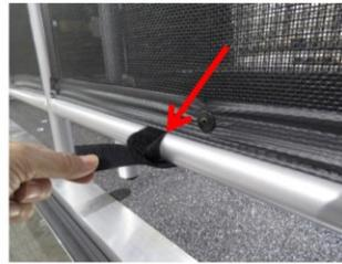
7. Remove the velcro straps (TIP: re-wrap them on the gates to ensure they aren't lost) that secure the end patio gates shut in the travel position.
