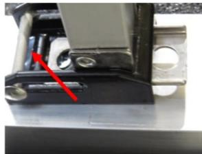
4. Insert the forward side of each retractable awning leg foot into the bracket first as shown above, then roll the pin forward over the rear edge of the foot (Tip: the pin locks the awning foot into the bracket).
