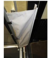
9. Lastly, slide on and fasten the fabric side protectors as shown.
