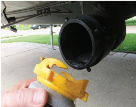
2. Open black waste holding tank valve and leave open to allow black tank to drain.
