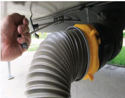
**NOTE:** To help ensure that debris does not clog tank sprayer orifices, use "TANK FLUSH" every time that the waste holding tank is emptied.
