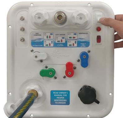
**NOTE:** LED indicator light below the pump switch will be lit if pump has power.
