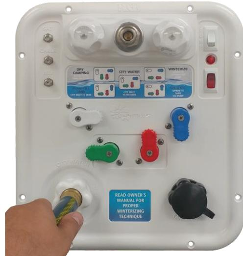
3. Place other end of hose in container holding water or sanitizing solution.
