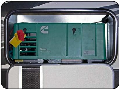
*Generator (If So Equipped) Is Located in the Forward, Off-Door Side Compartment of the RV.*
