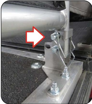
5. To secure the side patio gates vertically **INSERT** the safety pin *removed in step 3*, to the top-most position (*as shown*).
