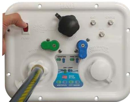
**NOTE:** LED indicator light below the pump switch will be lit if pump has power.
