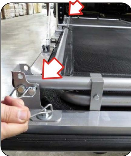
3. REMOVE the inside locking safety pins from the front & rear brackets.
