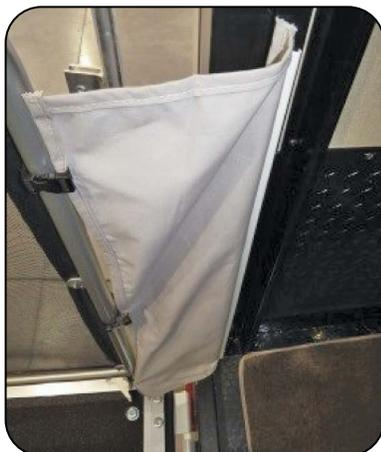
8. *Lastly*, slide the fabric side protectors into place between the unit and patio.
