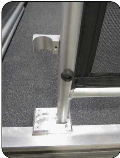
6. Swing the patio end gates from the open position, into the holder *as shown*.
