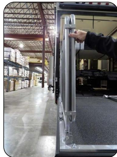
4. Carefully LIFT and SWIVEL the side patio gates to the vertical position.
