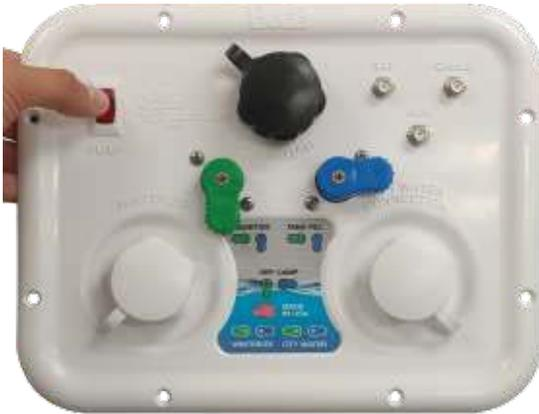
3. Push "**PUMP**" switch to turn pump on.
