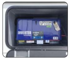
Generator (If So Equipped) Is Located in the Fwd, Off-Door Side Compartment
