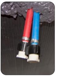
Low-Point Drain Valves located under the RV
