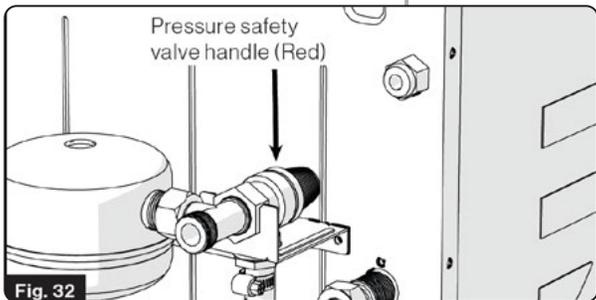
8. Inspect the pressure safety valve to ensure it has not been leaking (no water residue). See "Pressure Safety Valve Maintenance" for further inspection. (Fig. 32)
