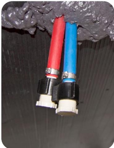
Low-Point Drains located under the RV
