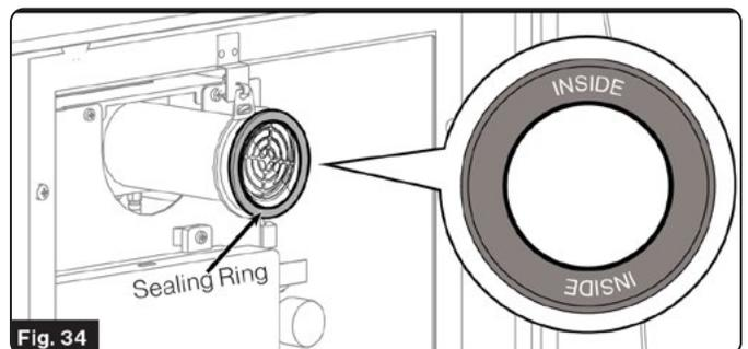
11. A sealing ring is assembled on the chimney. (Fig. 34)
