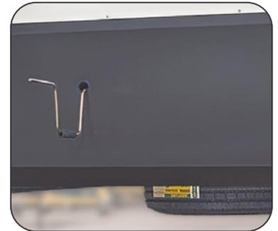
*Spare Tire, Access Hole & Crank Handle Extension*
