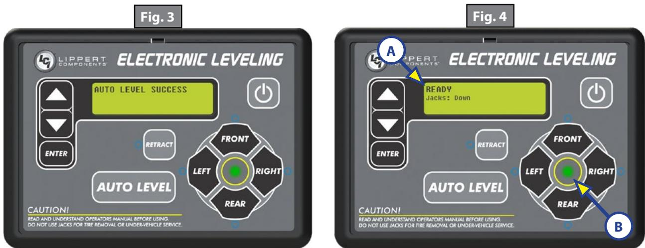
**NOTE:** If the AUTO LEVEL sequence does not perform as described, place the system in manual mode and test that the jacks operate correctly by pushing their coordinating buttons on the touch pad; i.e. "FRONT" button operates only the front jacks, etc.
