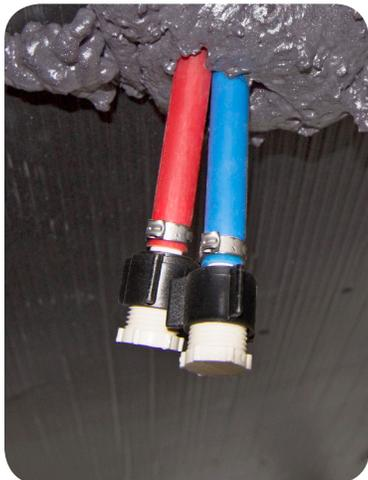
Low-Point Drains located under the RV
