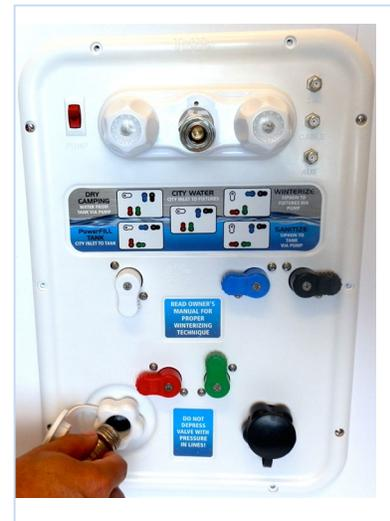
It is normal for some winterizing solution to exit inlet as hose is being disconnected.
