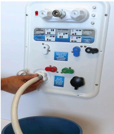
8. Push "**PUMP**" switch so that the light on switch is lit.
