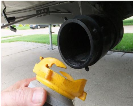
2. Open black waste holding tank valve and leave open. Allow tank to drain.
