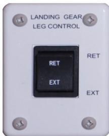
Typical LCI power landing leg control panel. Be aware that extend and retract indicate the travel direction of the legs, not the fifth wheel.
