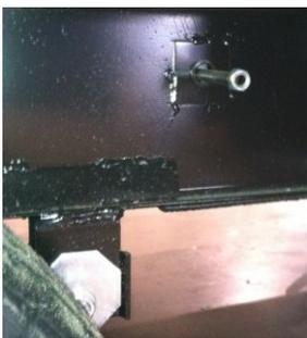
Typical 3/4" electric slideout system override.
