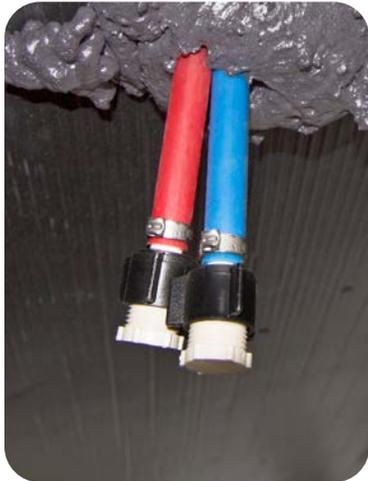
Low-Point Drains located under the RV
