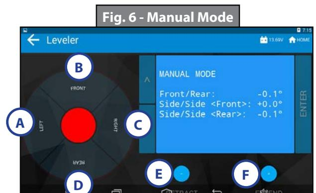
**NOTE:** If the rear jacks will not operate individually using the method described above, but they operate properly when Auto Level is performed, the Twist Prevention Protection system has locked out the operation to prevent damage to the frame of the trailer.
