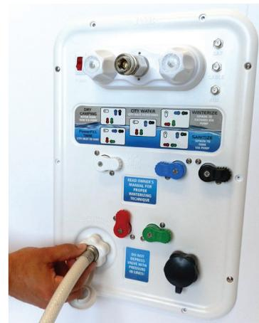
7. Turn water on. Fresh water tank should begin to fill.
