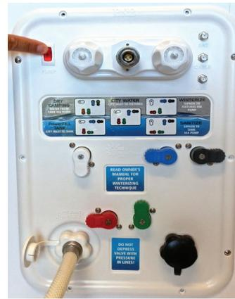
11. Pump should be running and winterizing solution should begin to flow through pump into plumbing lines and fixtures. (The pump will run when a plumbing fixture is open.)
