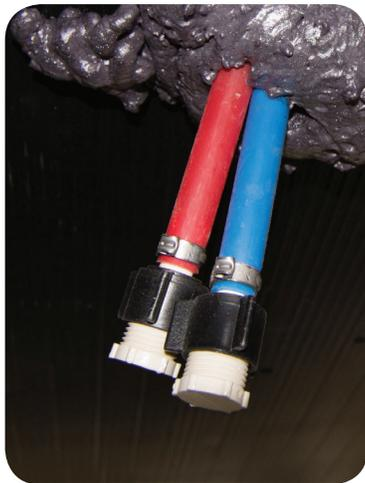
*Low-Point Drains located under the RV*
