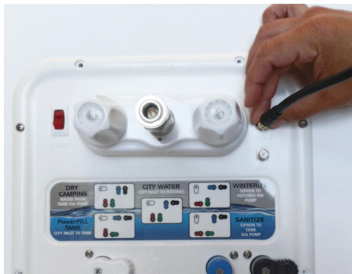
1. For cable TV connection, connect the threaded coax from the source to the **"CABLE"** connection.
