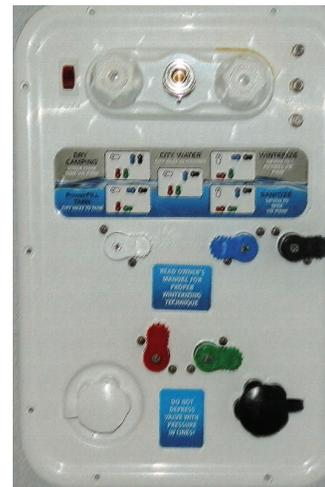
2. Open low point drain on RV to remove water in plumbing lines. Open both a hot and cold faucet to help drainage process.
