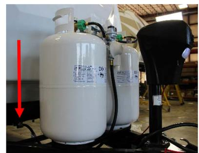
*Typical travel trailer double LP cylinder installation (arrow points to brass manifold fitting on trailer frame).*
