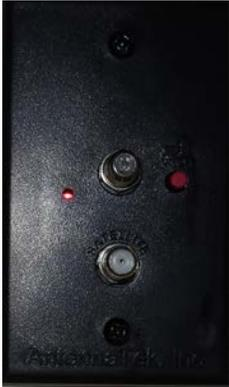
Typical TV signal booster, the ON/OFF red button is located on the right side of the face plate.
