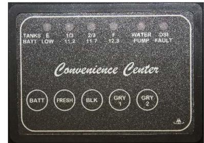
*Photo shows a typical monitor panel section, located on the Command Center inside the RV.*
