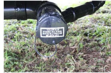
*Typical sewer outlet connection, located on the off-door side.*
