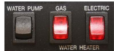
*Typical water heater and water pump ON/OFF switches, located on the Command Center inside the RV.*
