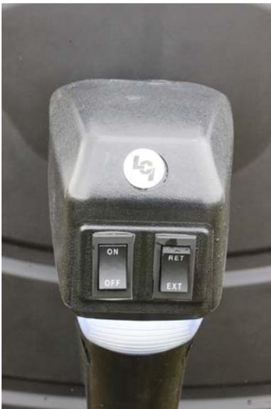
*Typical LCI power tongue jack control panel. Be aware that extend and retract indicate the travel direction of the leg, not the RV.*
