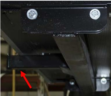
Typical rear hitch installation, shown on the 308BHTS.
