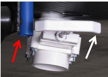
The white arrow indicates a typical fresh tank drain valve. The red arrow indicates a typical fresh water tank overflow tube/vent line (valve & drain locations vary by model).
