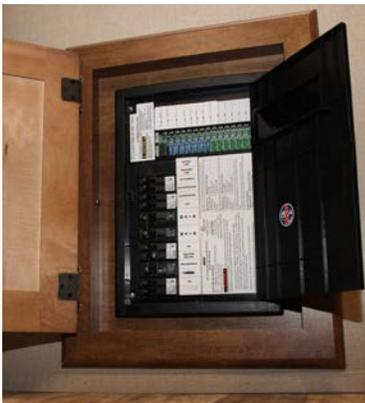
*Typical load center, shown in a Reflection 308BHTS.*
