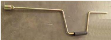
Typical electric slideout override manual crank handle.
