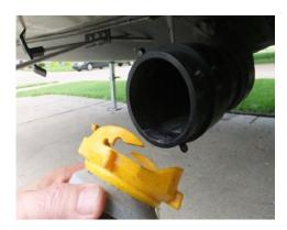
2. Open black waste holding tank valve and leave open. Allow tank to drain.
