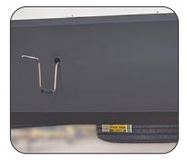
Spare Tire, Access Hole & Crank Handle Extension
