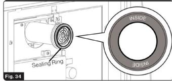
11. A sealing ring is assembled on the chimney. (*Fig. 34*) Inspect to make sure the seal does not have any cracks or breaks, and that it is in good condition. *Contact Furrion for replacement.*
