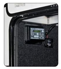
The Ground Control 3.0 LCD Touch Pad is located inside of the off-door side, forward compartment
