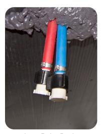
Low-Point Drains located under the RV
