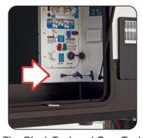
The Black Tank and Grey Tank Drain Valves (or dump valves) are located below the Nautilus P1 Water Panel.
