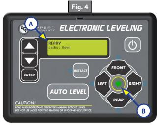
**NOTE:** If the AUTO LEVEL sequence does not perform as described, place the system in manual mode and test that the jacks operate correctly by pushing their coordinating buttons on the touch pad; i.e. "FRONT" button operates only the front jacks, etc.
