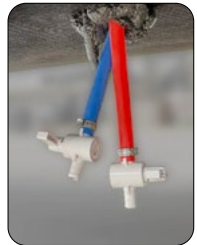
Low-Point Drain Valves located under the RV
