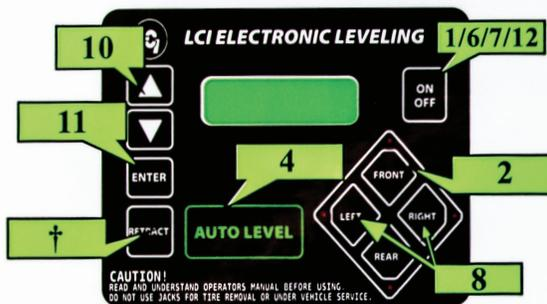
1. PRESS "ON/OFF" BUTTON TO TURN PANEL ON (DISPLAY READS "JACKS UP").
