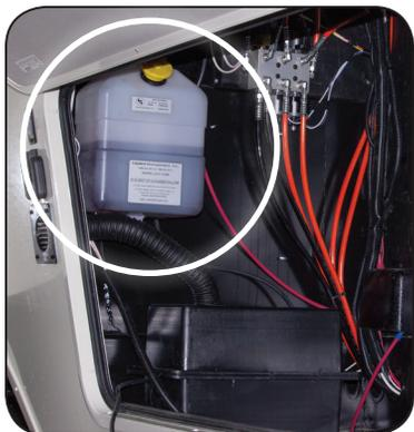
*The Hydraulic Fluid Reservoir is located in the Front Compartment. It supplies fluid to both the Hydraulic Landing Gear & the Hydraulic Slide Systems.*
