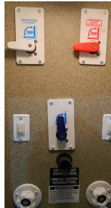
Typical valve positions for city water fill usage (connect hose to black inlet).
