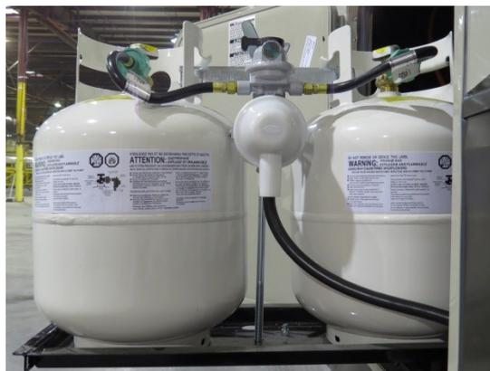
*This photo shows a typical configuration of the two main working 20 lb. cylinders located in the front off-door side compartment. (The front door side compartment contains a single spare cylinder that is not connected to the RV propane system; it is for storage purposes until needed only.)*
