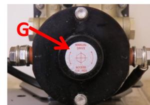
Typical protective seal, located on the end of the motor attached to the hydraulic reservoir.
