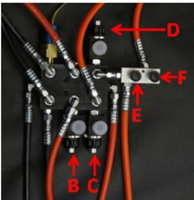
Typical hydraulic slide rooms and leveling legs override valves, generally located in the front facing compartment of the Solitude 369RL.
