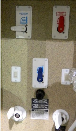
Typical valve positions for sanitization (connect hose to white city water fill inlet, located to the left of the white sewer tank flusher water inlet).
