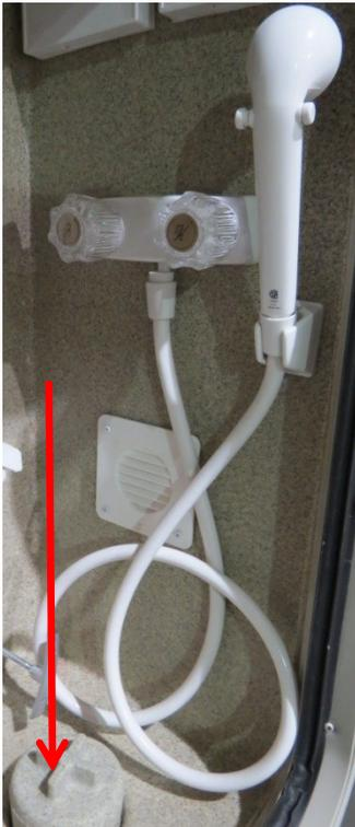
*Typical outside shower. Remove the drain plug at the water hose access (indicated by the arrow) to allow excess liquids to drain out of the compartment area. This drain plug is NOT designed to sit flush with the compartment floor when inserted in the travel (and storage) position.*
