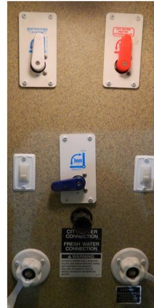
*Typical valve positions for winterization (connect hose to white city water fill inlet, located to the left of the white sewer tank flusher water inlet).*
