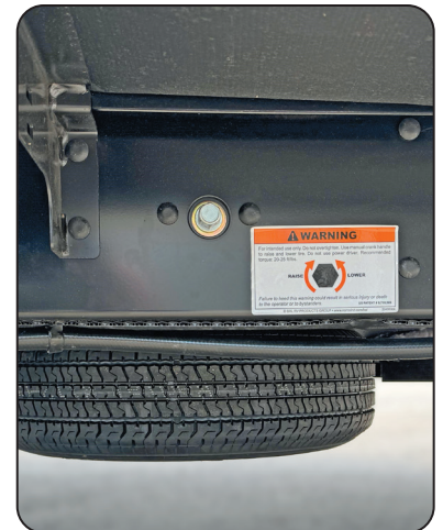
Use Crank Handle Extension to raise and lower tire.
